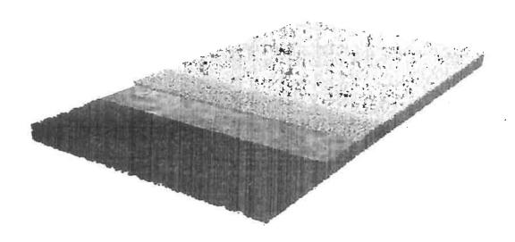
Double-layer sandwich system. Base layer made of recycled granules. Top layer made of polyurethane coating using premium CONIPUR EPDM Granules. Meets all important international standards, e.g. IAAF Specification, DIN V 18035-6, ASTM F2157-02 and EN 14877.
